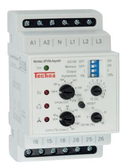
These relays monitor overvoltage, undervoltage, phase sequence, phase failure and phase voltage asymmetry in 3 Phase AC systems. The Montec-3PVM-Asym is for circuits without neutral and the Montec-3PVM-AsymN is for circuits with neutral.
